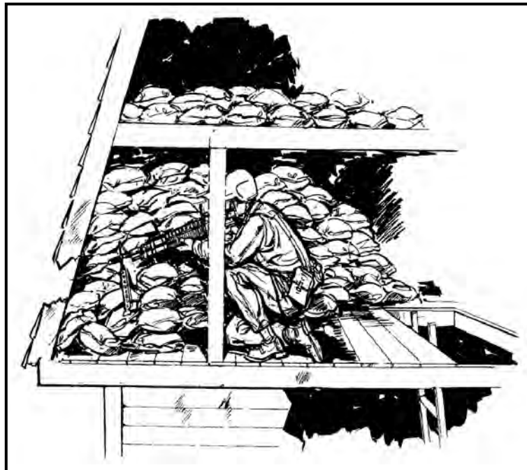
Figure 3-60. Firing platform built under roof.
