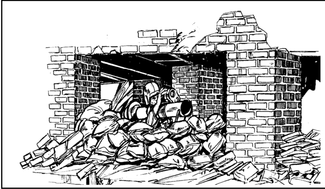
Figure 3-54. Prepared positions using a building for overhead cover.
